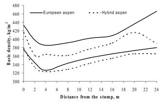
Figure. 3. Minimum and maximum values for the basic density of aspen wood
