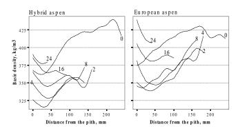
Figure 4. Basic density of hybrid (2137 specimens from 31 trees) and European aspen (2972 specimens from 44 trees) wood at different heights as a function of the distance from the pith. Line number represents the vertical location of the specimens as distance from the stump in metres
