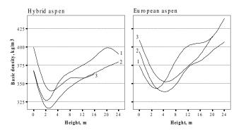
Figure 5. Basic density of hybrid and European aspen wood as a function of vertical position at pith (line 1), 40-mm-distance from the pith (2) and 80-mm-distance from the pith (3)
