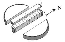
**Figure 1.** Manufacturing principle for specimens for annual ring width measurements (1) and basic density measurements (2). N shows to the north
